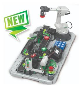
The VEX CTE Workcell kit is a construction system for a robotic arm, conveyors, and sensors.
